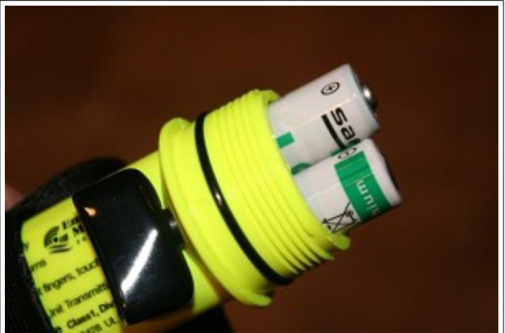
It is easiest to place the batteries into the shell at the same time. With black boot facing you, have positive battery on top and negative battery on bottom.
