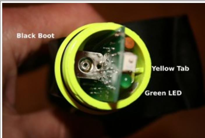
When placing circuit board into ALERT2 shell, make sure green LED on circuit board is facing opposite side of black boot that is on outside of shell.
