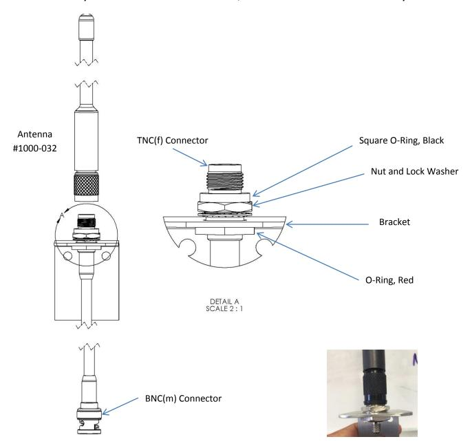
The coaxial cable has two different connectors. The BNC connector has a rotating lock that connects to the back of the ALERT2 Receiver. The other end has a TNC connector that attaches to the antenna mount. These instructions are for mounting the cable to antenna mount.
